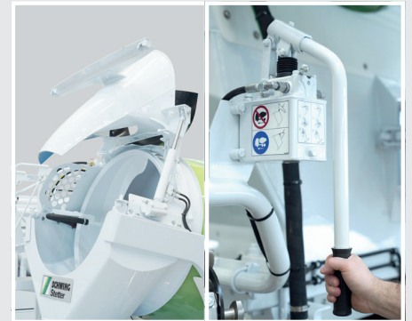
Hydraulically tilted filling hopper (allows high pressure cleaning of the mixing drum)
